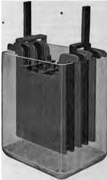
FIG. 812.—A Typical Storage Cell Enclosed in a Glass Jar. This cell represents one of the best-known makes of the Planté genus. With five plates, as shown, such a cell has a capacity of 80 ampere-hours, at 8 hours' discharge; of 70 ampere-hours, at 5 hours' discharge; of 60 ampere-hours, at 3 hours' discharge, with a discharge rate of 10 amperes in 8 hours; of 14 amperes in 5 hours, and of 20 amperes in 3 hours. The total outside dimensions of this cell are 5\frac{1}{4} \times 9\frac{1}{2} \times 11\frac{1}{4} inches; dimensions of each plate's active surface, 7\frac{1}{4} \times 7\frac{3}{4} inches.
